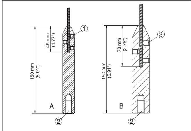
Fig. 20: Shortening the cable probe
