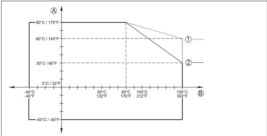
Fig. 28: Ambient temperature - process temperature, standard version
