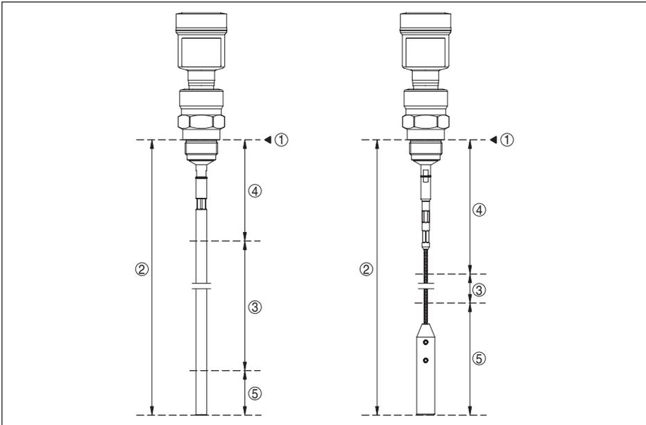
Fig. 25: Measuring ranges - NivoGuide 3100
