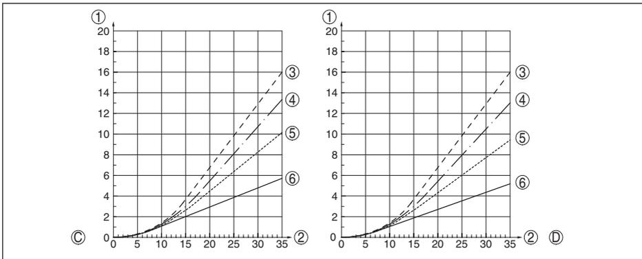
Fig. 22: Max. tensile load with sand and cement - Cable:  $\phi$  4 mm (0.157 in)
