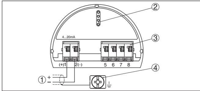
Fig. 10: Electronics and connection compartment - single chamber housing
