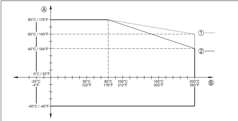
Fig. 29: Ambient temperature - process temperature, version with temperature adapter
