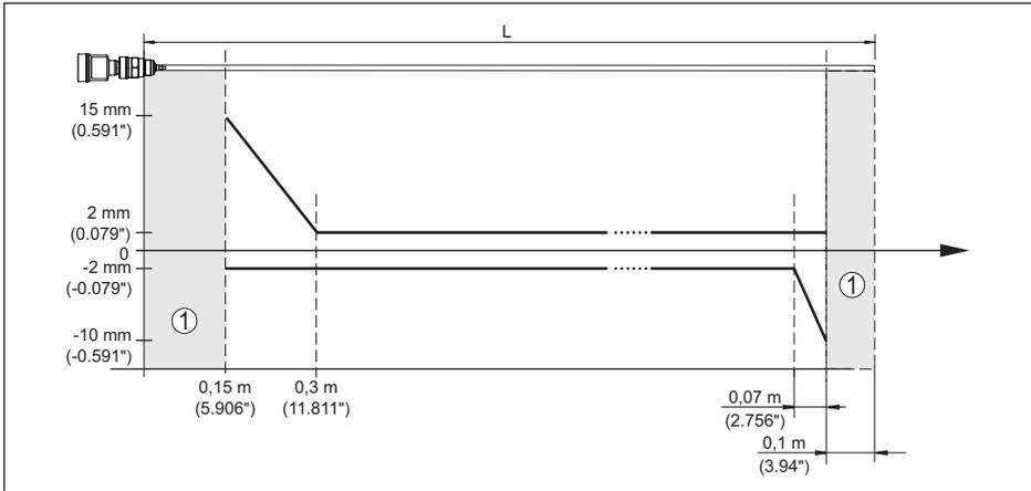
Fig. 26: Deviation NivoGuide 3100 in rod version
