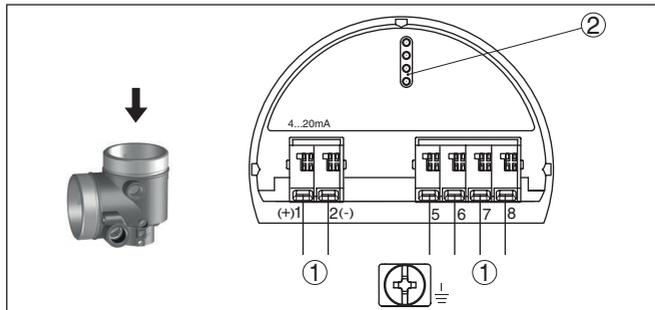
Fig. 11: Electronics compartment - double chamber housing
