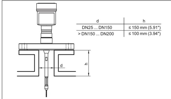
Fig. 5: Mounting socket
