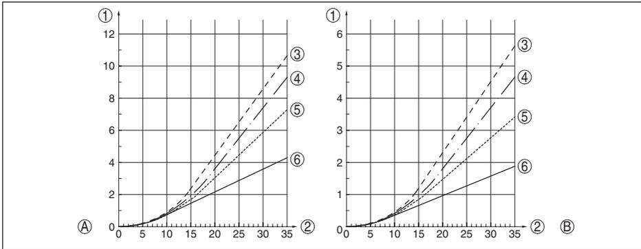
Fig. 21: Max. tensile load with cereals and plastic granules - Cable:  $\phi$  4 mm (0.157 in)
