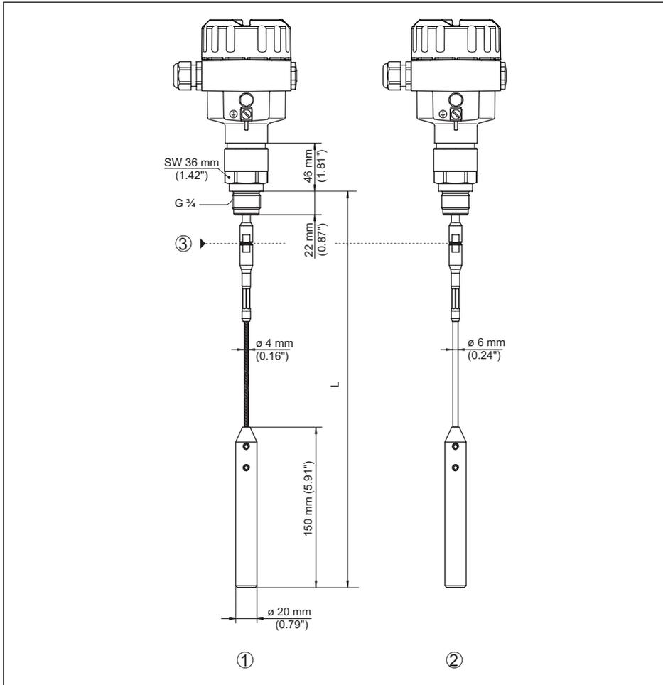
Fig. 32: NivoGuide 3100, cable  $\varnothing$  4 mm (0.157 in),  $\varnothing$  6 mm (0.236 in) threaded version with gravity weight (all gravity weights with thread M12 for eye-bolt)
