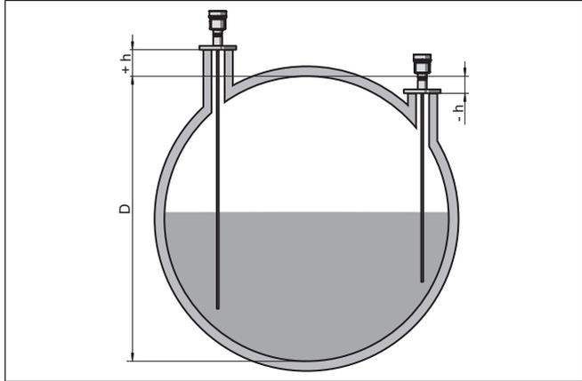
Fig. 16: Vessel height and socket correction value
