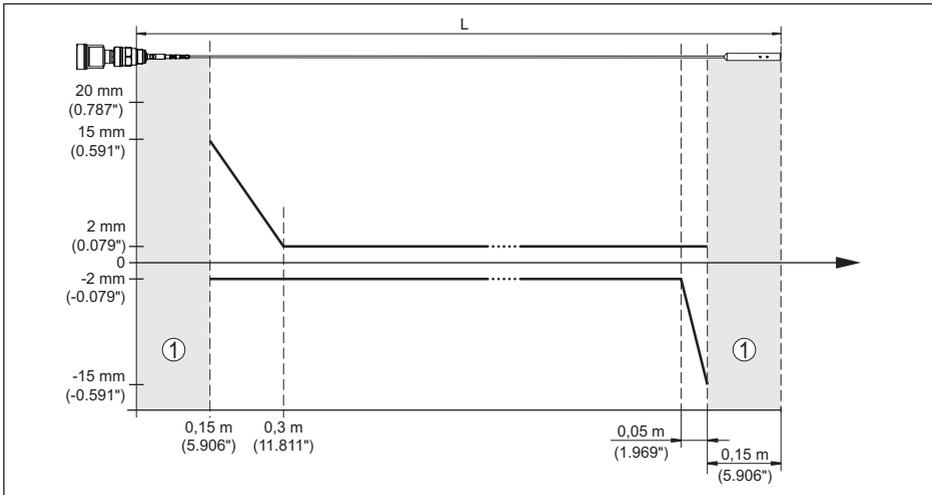
Fig. 27: Deviation NivoGuide 3100 in cable version
