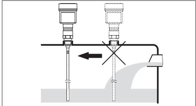
Fig. 7: Mounting of the sensor with inflowing medium
