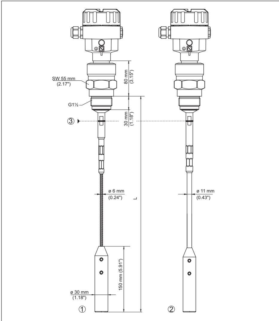
Fig. 33: NivoGuide 3100, cable  $\varnothing$  6 mm (0.236 in),  $\varnothing$  11 mm (0.433 in) threaded version with gravity weight (all gravity weights with thread M12 for eye-bolt)
