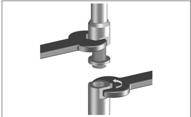
Fig. 19: Exchange cable or rod
