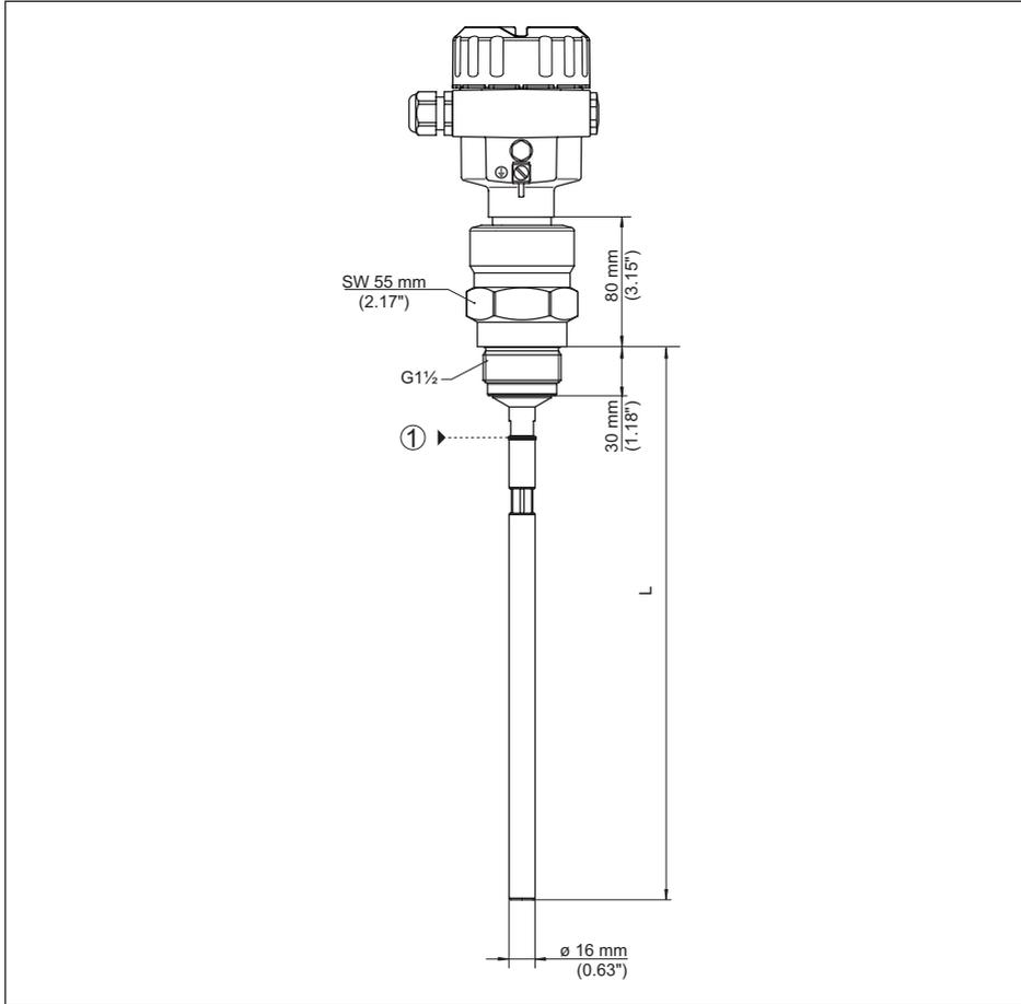
Fig. 34: NivoGuide 3100, rod  $\varnothing$  16 mm (0.63 in), threaded version
